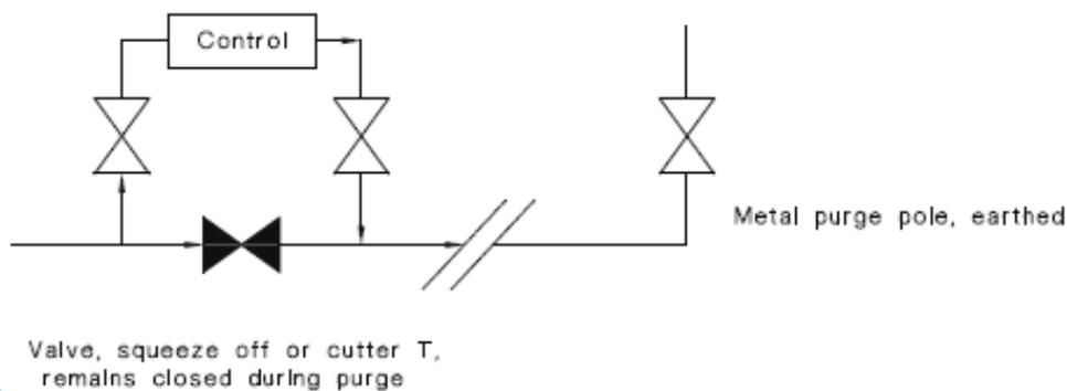
FIGURE E2 GRADUAL PURGE FOR MAINS AND SERVICES ABOVE 100KPA - BYPASS CONNECTION MAY MAKE USE OF CURRENT OR FUTURE SERVICE T'S
