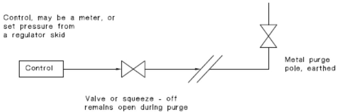
FIGURE E3 GRADUAL PURGE FOR MAINS AND SERVICES ABOVE 100 KPA— CONTROL CONNECTION MAY MAKE USE OF A METERING OR PRESSURE REGULATION SKID
