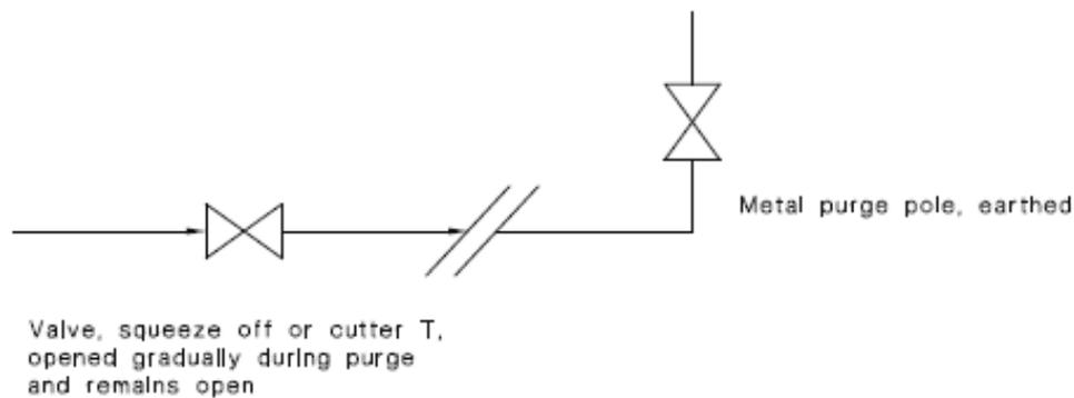
FIGURE E1 STAGED PURGE FOR MAINS AND SERVICES BELOW 100 KPA
